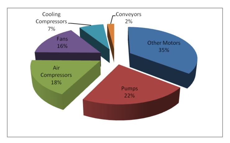
Disaggregation of motor electricity consumption by end-use, in the EU Industrial sector
